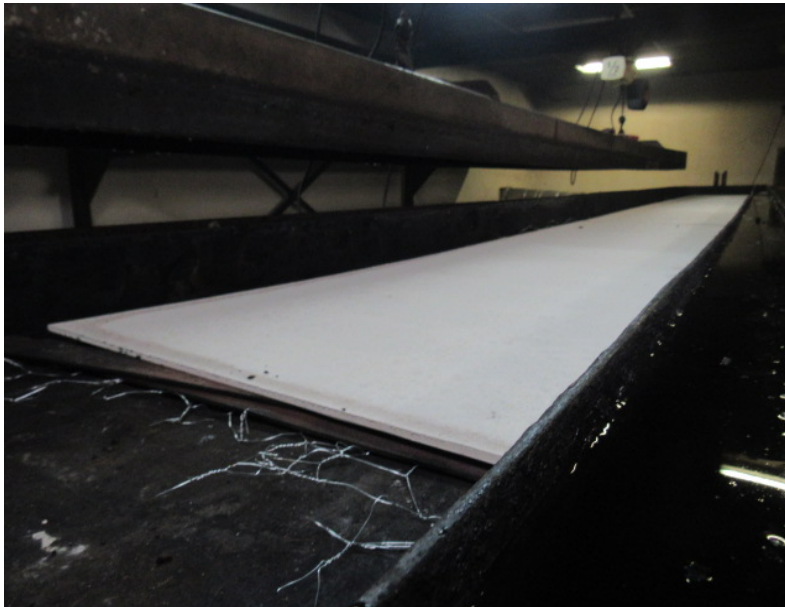
Photo No. 2 Unexposed Surface of the Test Specimen (Pre-test)
